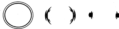
Fig. 8.17. X-ray scattering patterns of PE, as registered for the isotropic part ( left ), the center of the shoulder ( center ) and the neck ( right ) of a cold-drawn sample. The two reflections in the isotropic pattern are to be assigned to the 110- and the 200-lattice planes of orthorhombic polyethylene. The third reflection with a larger lattice plane spacing emerging in the textured patterns is due to another metastable crystalline phase which forms during drawing [85]
