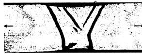
Fig. 8.2. Formation of shear bands at the begin of necking, observed for a sample of PC. The arrows indicate the direction of the applied tensile stress. Micrograph obtained by Morbitzer [82]
