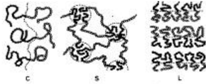
Fig. 8-16 Arrangement of A-blocks with A-units ● and B-blocks with B-units ○ in diblock copolymers A_n-B_m (C, L) and in triblock copolymers A_{n/2}-B_m-A_{n/2} (S) [8]. Note that n and m in this figure refer to the respective space requirements and not to the amounts of monomeric units. C: Compatibilizer at the phase boundary - - - between A-polymers and B-polymers. S: Spherical A-domains in a continuous B-matrix ( m \ll n ). L: Lamellae with A-layers and B-layers ( n = m ).
