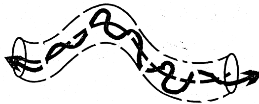
Fig. 6.10. Modelling the lateral constraints on the chain motion imposed by the entanglements by a 'tube'. The average over the rapid wriggling motion within the tube defines the 'primitive path' ( continuous dark line )
